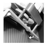
Pull out the pin on top of the sharpening device in direction of arrow and move the sharpening device over the edge of the thickness plate.
