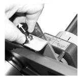
Move the sharpening device with the pin pulled out to the front in the direction of the blade (direction of arrow), so that the pin is engaged in the hole of the thickness plate.
